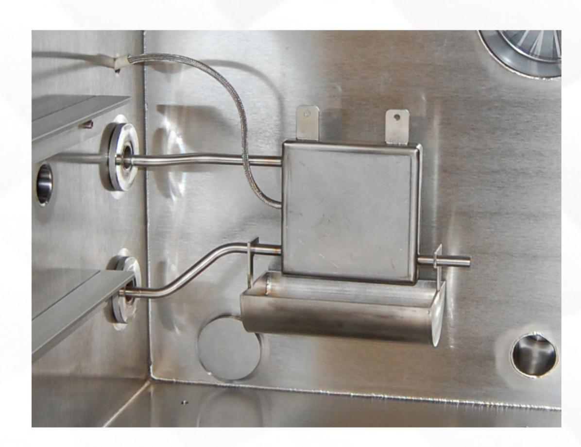
When testing spacecraft or equipment under the vacuum and thermal conditions of space, the scavenger plate helps absorb any outgassing from materials inside the chamber.
