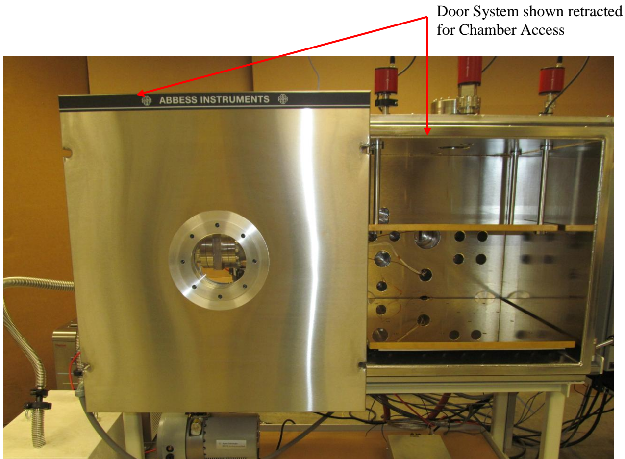
Figure 3 – View of Thermal Vacuum Chamber (Door Open)
