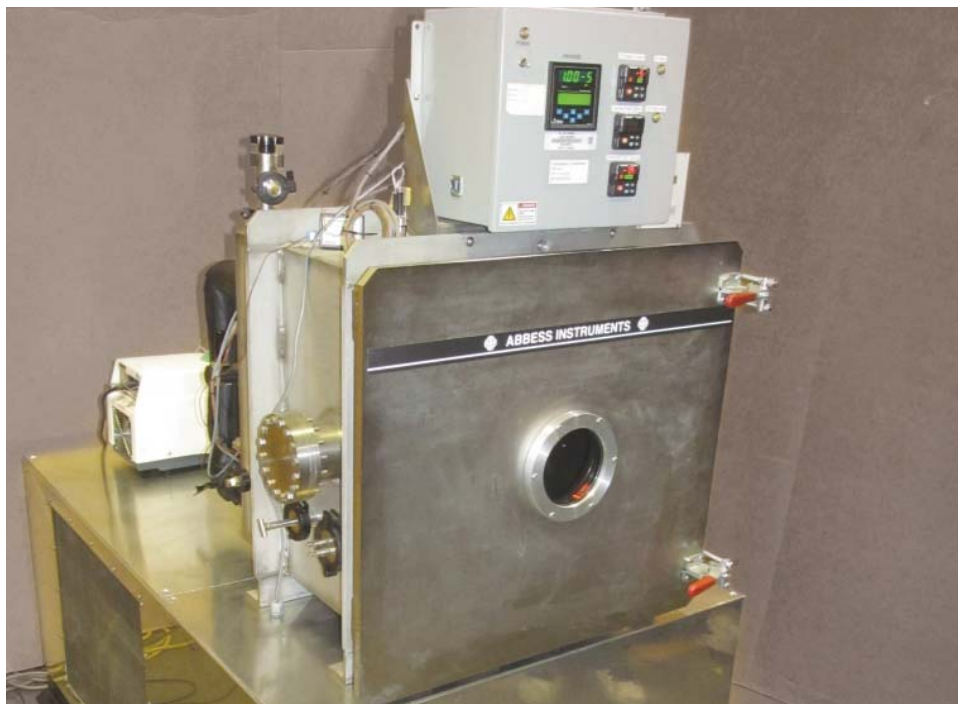
Custom designed thermal platen in high vacuum chamber system with -80°C cascade refrigeration.
